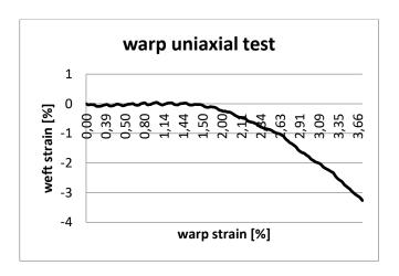
Figure 4. Transversal deformation, uniaxial test, warp loading.
