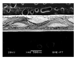
Figure 7. Microscopic photo of the section, the cut is parallel to the weft direction.
