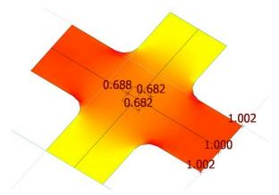
Figure 9. FEM analysis to approximate the stress level in the measured area.
