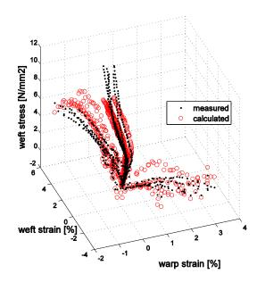
Figure 10. The general result of the parameter identification for the weft direction.
