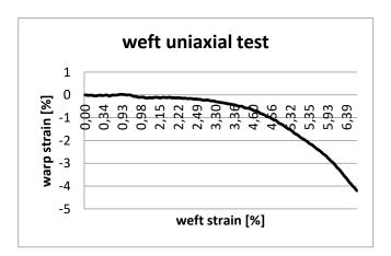
Figure 5. Transversal deformation, uniaxial test, weft loading.
