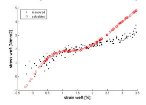
Figure 13. The uniaxial result of the parameter identification for the weft direction.
