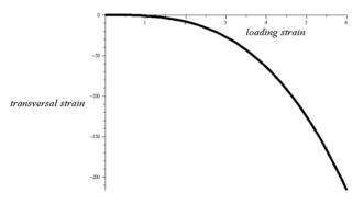
Figure 6. Calculated transversal deformation for uniaxial loading.
