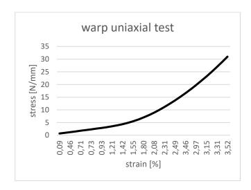
Figure 1. Measured stress, a typical stress-strain curve of a uniaxial tensile test in the warp direction.
