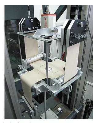
Figure 8. The bidirectional testing equipment.
